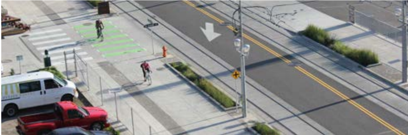
Intersection crossing markings can be used at signalized intersections or high volume minor street and driveway crossings, as illustrated above.
